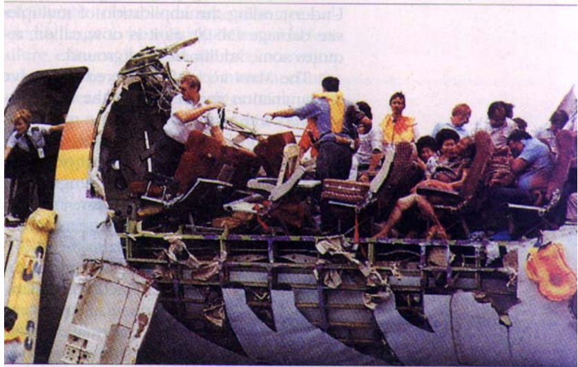
Figure 1 – Aloha Airlines Boeing 737 experienced catastrophic “un-zipping” of large portions of the fuselage in 1988 due to multi-site cracks in the skin joints
